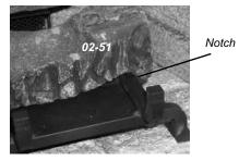
Position Log <u>02-53</u> across the cutouts in Logs 02-75 and 02-51 with the notch on the left side of the log fitting into the 2nd grate
